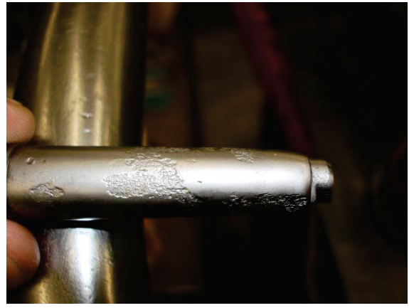
Medium-Sized Non-Nitrided Core after 55000 shots
