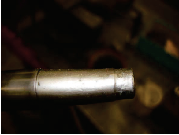
Medium-Sized Non-Nitrided core after 35,000 shots
