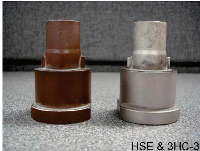
Side by side HSE CVD @ 50,000 & 3HC Different PVD @ 50,000
