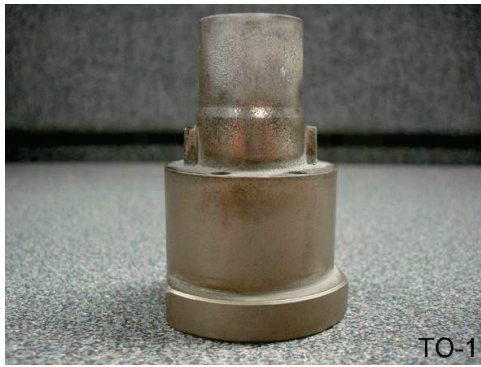
TD+ High Temperature Coating @ 50,000 shots
