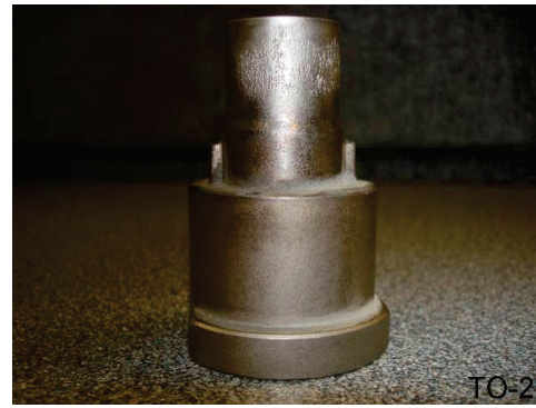
TD+ High Temperature Coating @ 20,000 shots
